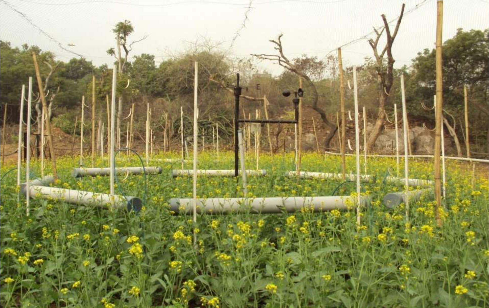
**Free Air Carbon dioxide enrichment (FACE) facility built in the campus of Jawaharlal Nehru University. Mustard (*Brassica*) plants are grown inside two FACE Rings maintained at elevated CO<sub>2</sub> (600 ppm)**
