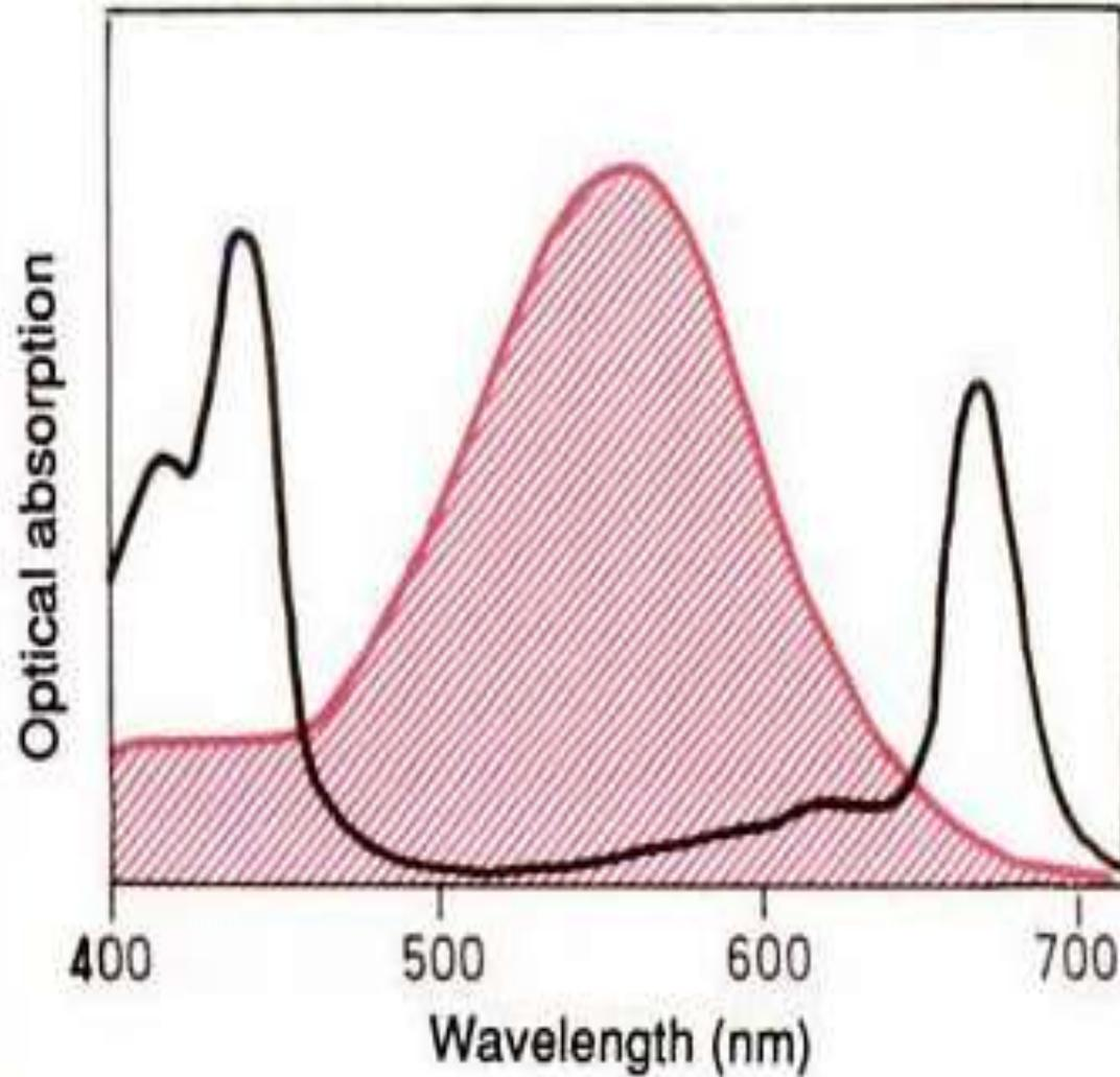
The absorption spectrum of chlorophyll a superimposed on the absorption spectrum of membranes containing bacteriorhodopsin (shaded). Chlorophyll's absorption peaks fit neatly on either side of bacteriorhodopsin's
