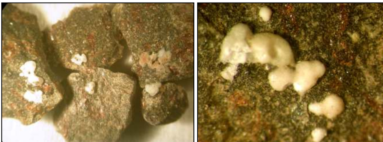
Secondary Ca/Mg/Fe carbonates formed by reacting \text{CO}_2 and Picrite (Western DVP)
